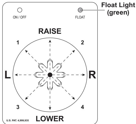
From the center position, the control lever can be moved in one of eight (8) directions to control various movements of the snowplow blade. To change from one movement of the blade to another, the control lever must be moved back to the center position before selecting the desired function. Whenever the lever is released, it should spring back into the center position to stop any blade movement.
